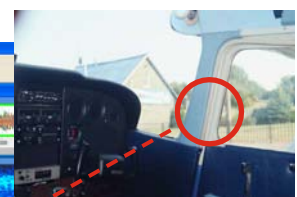
Fig. 10 Side window as source; 2 to 6 kHz
