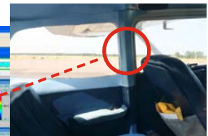
Fig. 9 Source at B-pillar; 2 to 6 kHz
