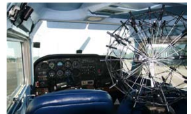
Fig. 3 Array position inside cavity
