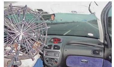
Fig. 3 Array position inside the cavity
