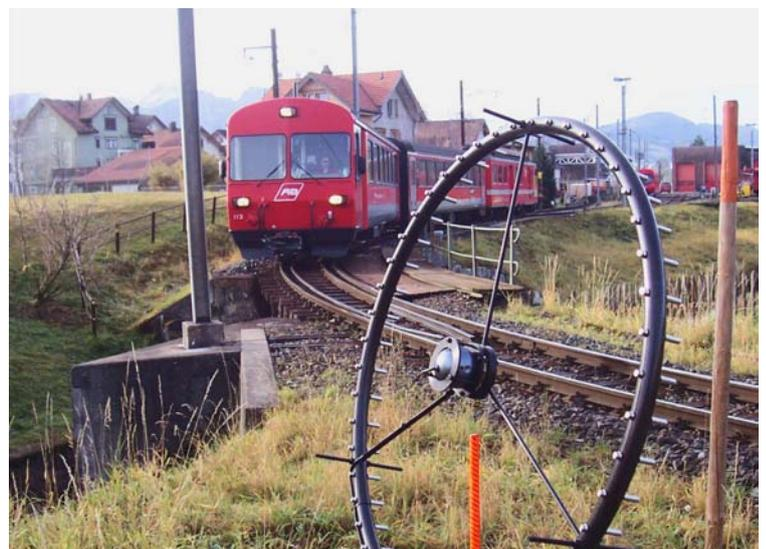
Fig. 8 Appenzeller Train passing by at measurement set up of the Acoustic Camera
