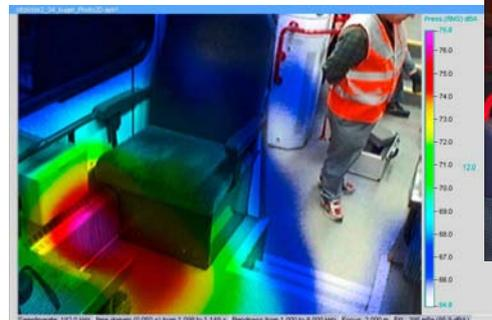
Fig. 5 Acoustic Photo 2D of emission from heater
