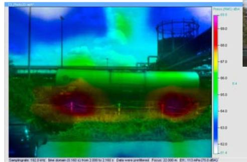
Fig. 3 Wheel emission at rolling tank wagon
