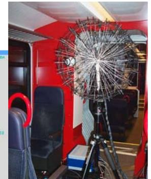
Fig. 6 Set up inside train
